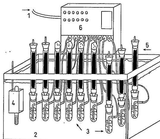
Fig. 1. Diagram of the inoculation device used for solid-state fermentation: 1, air inlet; 2, temperature-controlled vessel; 3, humidifier; 4, heating system; 5, reactors; 6, air-flow control
