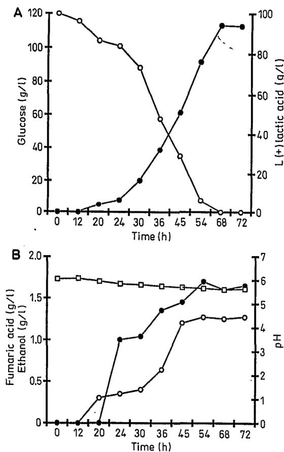
Fig. 4A, B. Kinetics of L(+)-lactic acid production by *R. oryzae* NRRL 395 in submerged culture. A Changes in glucose uptake (○) and L(+)-lactic acid formation (●) with time. B Changes in pH (□), fumaric acid (○) and ethanol formation (●) during fermentation
