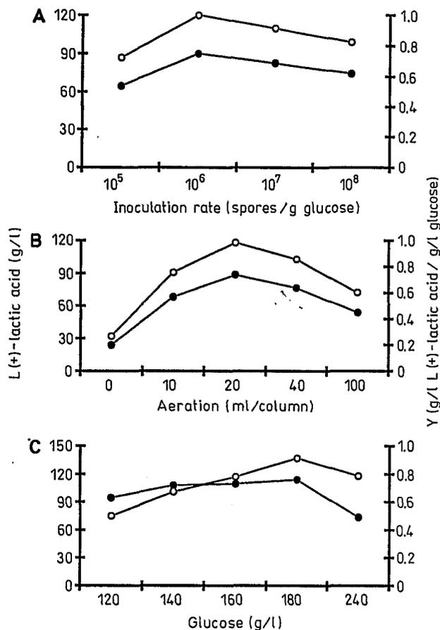
Fig. 2A-C. Effect of the various culture conditions on L(+)-lactic acid production (○) and productivity (●) *R. oryzae* NRRL 395 in solid-state fermentation. A Effect of inoculation rate. B Effect of aeration rate. C Effect of glucose concentration
