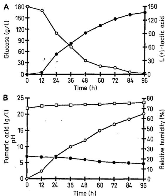
Fig. 3A, B. Kinetics of L(+)-lactic acid production by *R. oryzae* NRRL 395 in solid-state fermentation. A Changes in glucose uptake (○) and L(+)-lactic acid formation (●) with time. B Changes in relative humidity (□), pH (●) and fumaric acid formation (○) during fermentation
