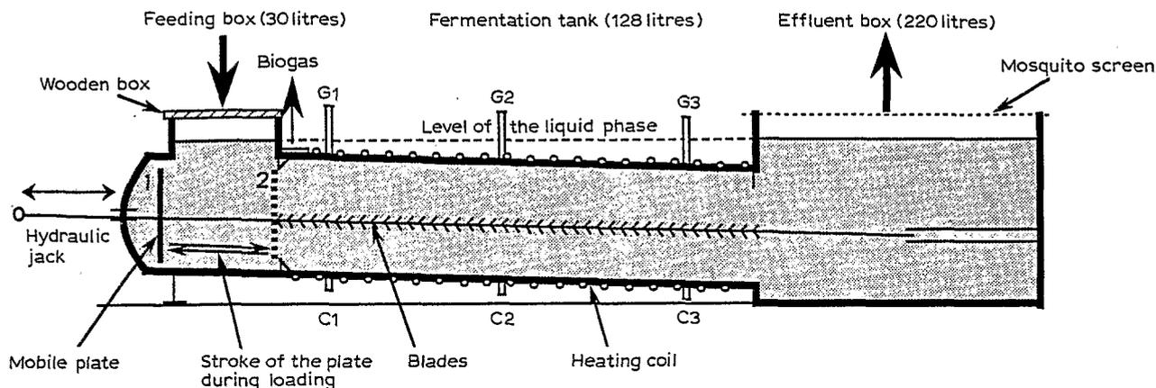
Fig. 1. 'Transpaille' fermenter — longitudinal cross-section. G1, G2, G3, Gas sampling points; C1, C2, C3, liquid sampling points; 1, position for loading; 2, position during fermentation. See text for detailed explanation.
