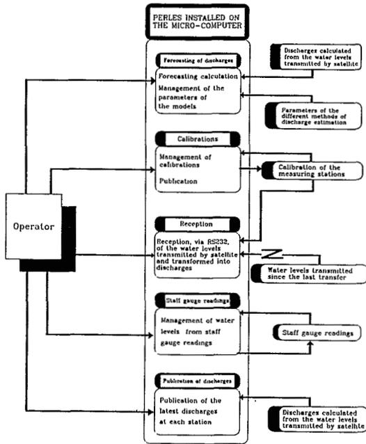
Fig. 4. Flow diagram of the PERLES software in the microcomputer used for forecasting calculations.
