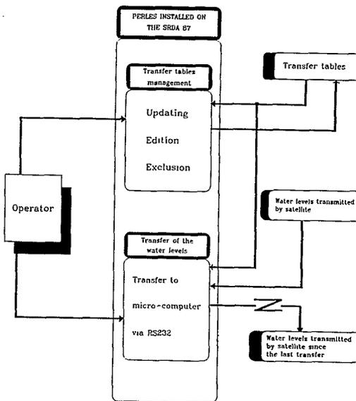
Fig. 3. Flow diagram of the PERLES software at the data reception station.
