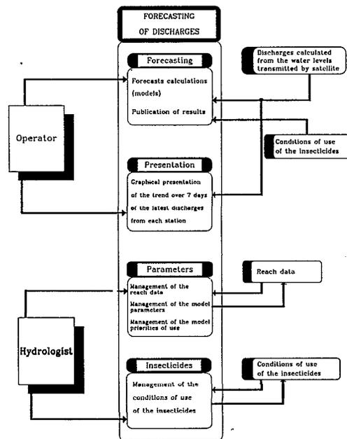
Fig. 5. Flow diagram of the forecasting part of the PERLES software.
