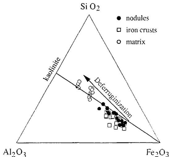
Fig. 3. Preferential leaching of iron with regard to aluminum during the iron crust dismantling.
