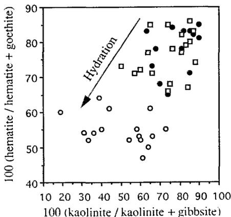
Fig. 2. Simultaneous increase of goethite and gibbsite in the dismantling facies of iron crust consisting of hematite and kaolinite as a function of the hydration increase.
