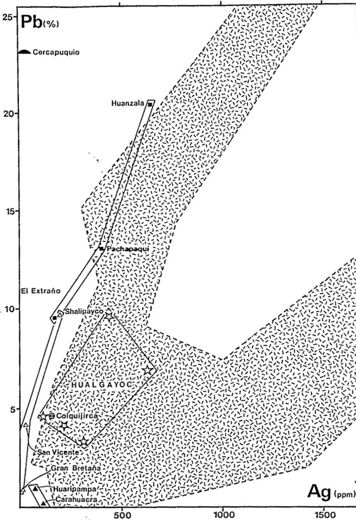
Fig. 5. Ag(ppm)-Pb(%) diagram (Symbols as in Fig. 2, but for each deposit the plotted data correspond to the average of ore analyses; the *dashed area* is the envelope of the data from the Cenozoic skarn and vein deposits, Lara et al. 1983)
