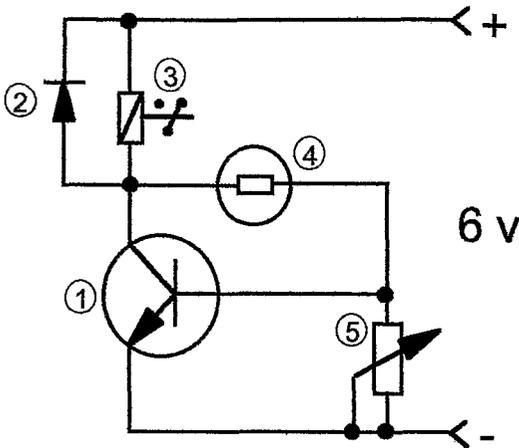
Fig. 2. Circuitry of the electronic light-switch. 1: Transistor 2N222, 2: Diode 1N4148, 3: Electromagnetic switch 6V/100 Ohms, 4: Photoresistance LDR05, 5: Adjustable resistance 4.7 Kohms.
