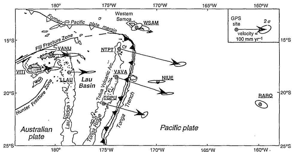
uncertainty in each velocity vector is represented by a 2σ (~86% confidence) error ellipse. The aspect ratio and orientation of these ellipses mainly reflects the fact that GPS satellite orbital errors are larger across-track than along-track. The velocities of the Tongan stations, which range from 164 ± 5 mm yr<sup>-1</sup> at Tongatapu (TGPU) to 240 ± 11 mm yr<sup>-1</sup> at Niuatoputapu (NTPT), manifest the rate at which the Pacific plate is subducting.
