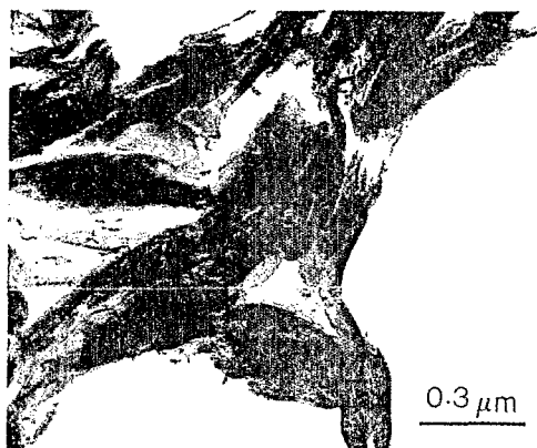
FIG. 6. Transmission electron micrograph of an aggregate of silhydrite.
