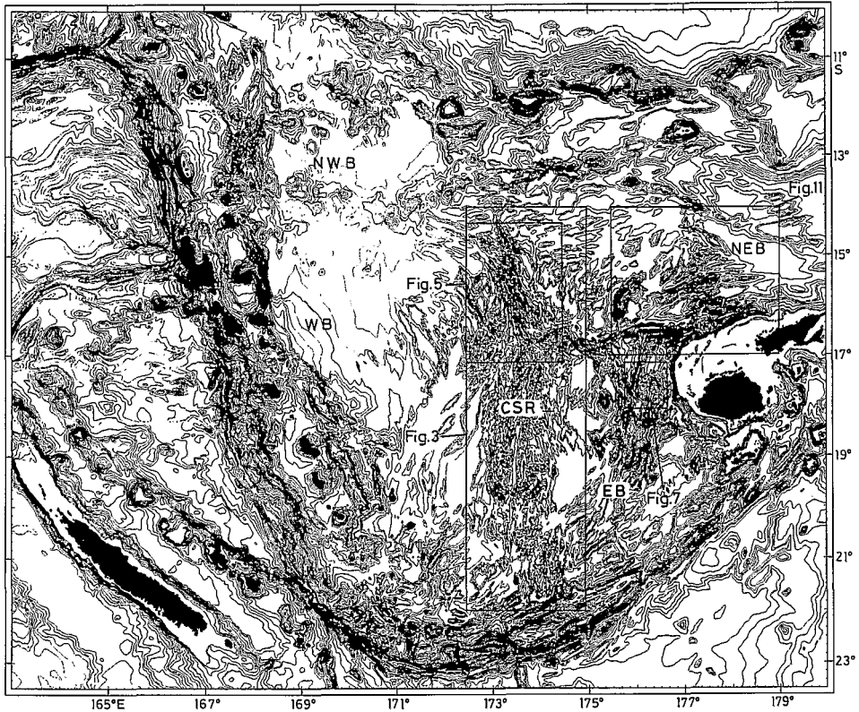
FIGURE 4.2. Bathymetric map of the NFB. This map results from a compilation (J.P. Mazé) of all multibeam data existing on the NFB (SEAPSO, Proligo, STARMER, Multipso cruises). The contour interval is 200 m. CSR: central spreading ridge; WB: western basin; E: eastern basin; NWB: northwestern basin; NEB: northeastern basin. Locations of Figs. 4.3, 4.5, 4.7, and 4.11 are shown.
