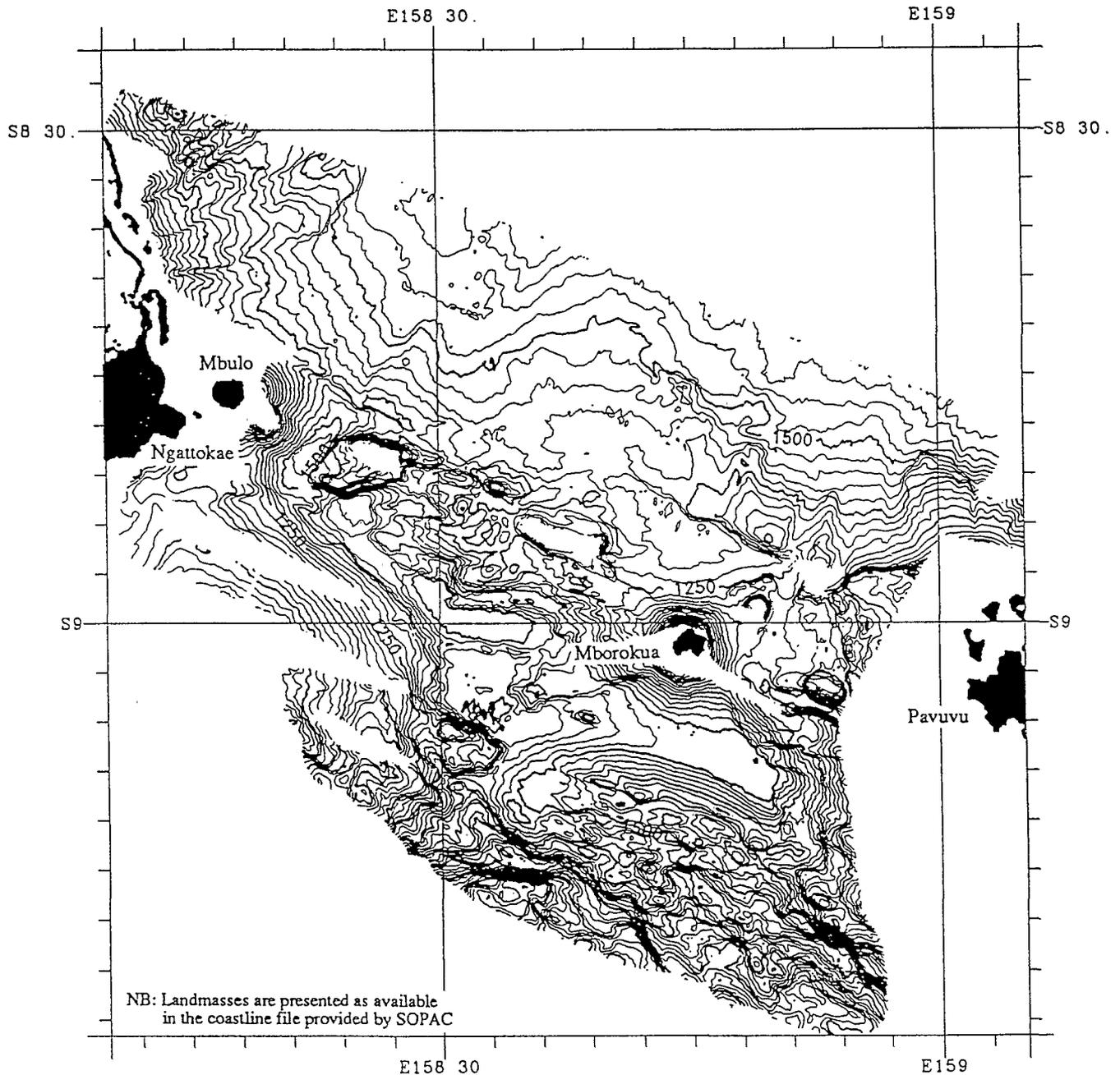
**Fig. 2** MultiBeam (SIMRAD EM12) map of the Mborokua Basin. Isobath interval = 50 m. In black, the emerged lands
