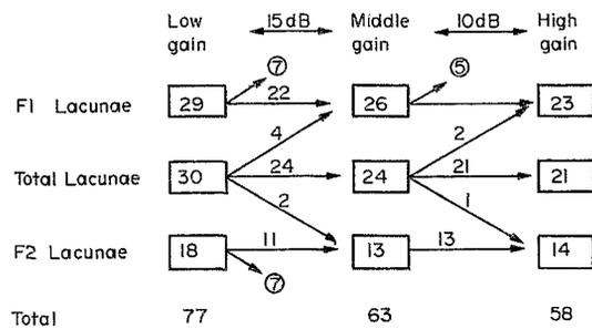
Fig. 4. Influence of the gain of the receiver. Numbers in squares are those of observations of *F*-lacunae. Circles indicate ionograms without appearance of lacunae. Arrows show how the appearance of the ionograms changes when increasing the gain.
