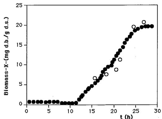
**Figure 6.** Dry biomass concentration,  $X$ , variation with time for the growth of *A. niger* No. 10 on Amberlite IRA-900 with initial sucrose solution concentration of 90 g/L and  $Q = 1.8 \text{ min}^{-1}$ . (●) Estimated values from pressure drop ( $\Delta P/L$ ); (○) experimental values. Fermentor size 4 cm i.d. and bed height 15 cm.
