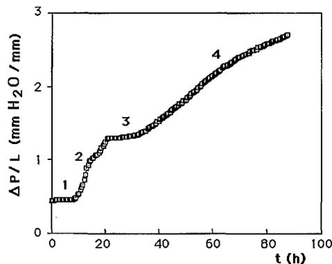
**Figure 9.** Variation of pressure drop ( $\Delta P/L$ ) with time in the fermentation of *A. niger* No. 10 on cane bagasse.  $S_i = 130$  g/L,  $Q = 3.5$  min $^{-1}$ , initial water content = 70%.
