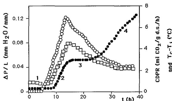
**Figure 8.** Variation of pressure drop,  $\Delta P/L$  ( $^{\circ}$ ); carbon dioxide production rate, CDPR (o); and temperature difference between fermentor center and the inlet temperature,  $T_c - T_i$  ( $\square$ ), with time in the fermentation of *A. niger* ANH-15 on wheat bran.  $Q = 2.7$  min $^{-1}$ , initial water content = 50%. Fermentor size 4 cm i.d. and bed height 15 cm.
