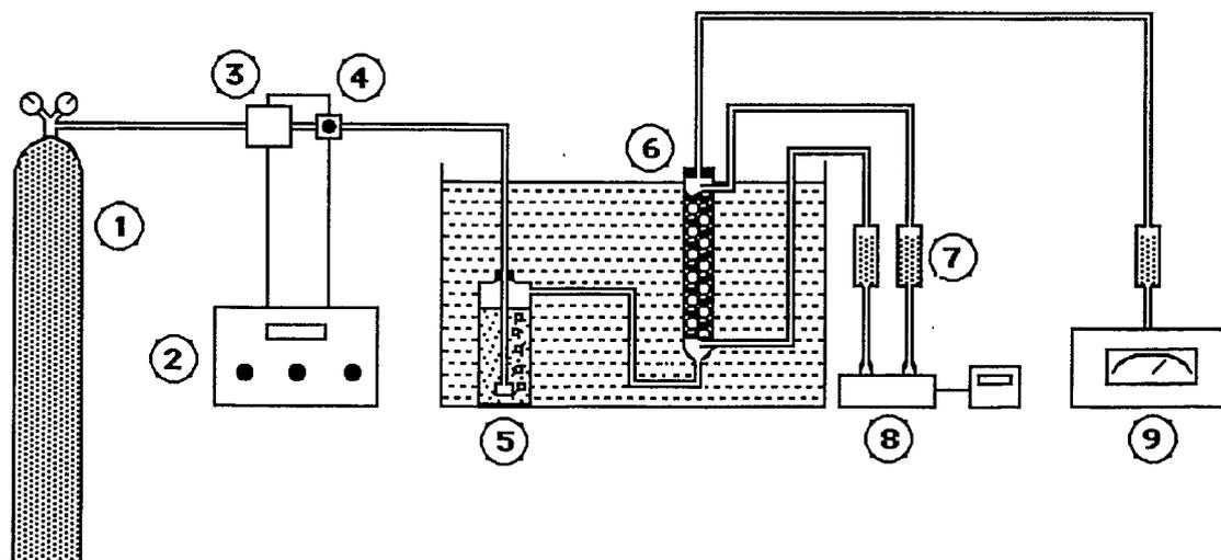
**Figure 1.** Experimental apparatus: 1, air supply; 2, flow controller; 3, flow meter; 4, control valve; 5, humidifier; 6, fermentor; 7, gas dehumidifier; 8, pressure transducer; 9, infrared  $\text{CO}_2$  analyzer.
