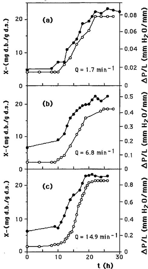
**Figure 4.** Dry biomass concentration  $X$  (●) and pressure drop ( $\Delta P/L$ ) (○), variation with time for the growth of *A. niger* No. 10 on Amberlite IRA-900 for different air-flow rates,  $Q$ , for initial sucrose solution concentration of 65 g/L. (a)  $Q = 1.7 \text{ min}^{-1}$ ; (b)  $Q = 6.8 \text{ min}^{-1}$ ; (c)  $Q = 14.9 \text{ min}^{-1}$ .
