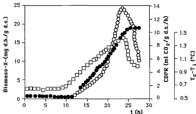
**Figure 7.** Variation of dry biomass concentration,  $X$  ( $^{\circ}$ ); carbon dioxide production rate, CDPR (O); and temperature difference between fermentor center and the inlet temperature,  $T_c - T_i$  ( $\square$ ), with time for the growth of *A. niger* No. 10 on Amberlite IRA-900.  $S_i = 90$  g/L and  $Q = 1.8$  min $^{-1}$ . Fermentor size 4 cm i.d. and bed height 15 cm.
