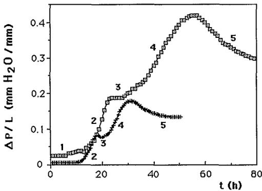
**Figure 2.** Variation of pressure drop ( $\Delta P/L$ ) with fermentation time for the growth of *A. niger* No. 10 on Amberlite IRA-900 at: (—○—)  $Q = 2.1 \text{ min}^{-1}$ ; initial sucrose solution concentration,  $S_i = 65 \text{ g/L}$ ; (—□—)  $Q = 4 \text{ min}^{-1}$ ,  $S_i = 200 \text{ g/L}$ .
