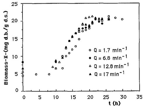
**Figure 3.** Dry biomass concentration  $X$  variation with time for different air-flow rates for the growth of *A. niger* No. 10 on Amberlite IRA-900.
