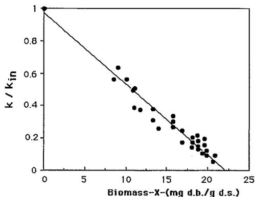
**Figure 5.** Variation of the relative permeability,  $k/k_{in}$ , with dry biomass concentration,  $X$ .
