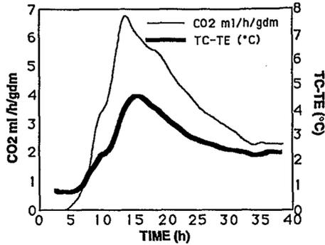
FIGURE 3. CO<sub>2</sub> production rate and temperature difference as a function of time.
