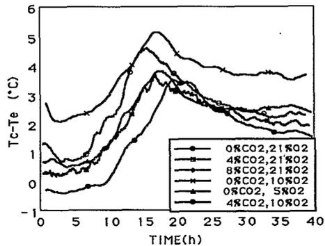
FIGURE 12. Temperature gradient as related to different gas environments.
