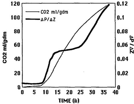
FIGURE 4. Evolution of pressure drop and the integrated value of CO<sub>2</sub> with time
