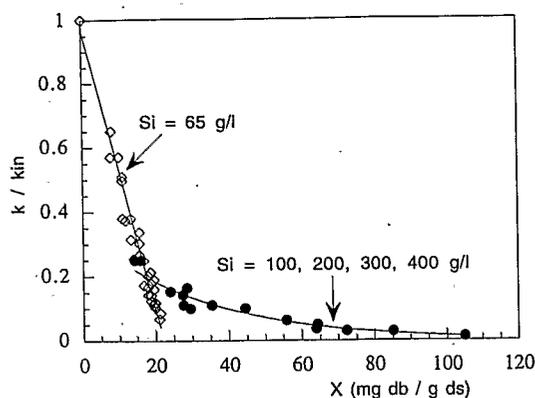
Fig. 4. Variation of the relative permeability,  $k/k_{in}$  ( $\bullet$ ) with dry biomass concentration ( $X$ ) for different initial sucrose solution concentration,  $S_i = 100$  g/litre; 200 g/litre; 300 g/litre; 400 g/litre. ( $\diamond$ ) Relation of  $k/k_{in}$  and with biomass for  $S_i = 65$  g/litre.<sup>10</sup>
