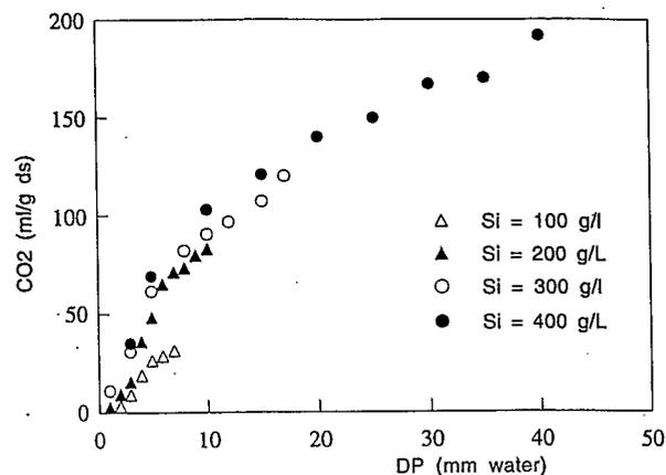
Fig. 5. Variation of evolved  $CO_2$  with pressure drop ( $DP$ ) for different initial sucrose solution concentration,  $S_i = 100$  g/litre; 200 g/litre; 300 g/litre; 400 g/litre.
