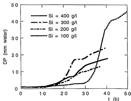
Fig. 3. Variation of pressure drop ( $DP$ ) with time for the growth of *A. niger* No. 10 on Amberlite IRA-900 for different initial sucrose solution concentrations,  $S_i = 100$  g/litre; 200 g/litre; 300 g/litre; 400 g/litre.
