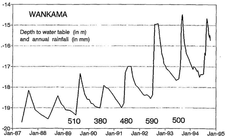
Fig. 6. Piezometric fluctuation in Wankama (1987–1994) with annual rainfall.
