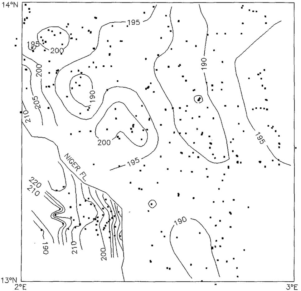
Fig. 2. Monitoring network and piezometric map of the degree square in September 1993 (curve every 5 m).
