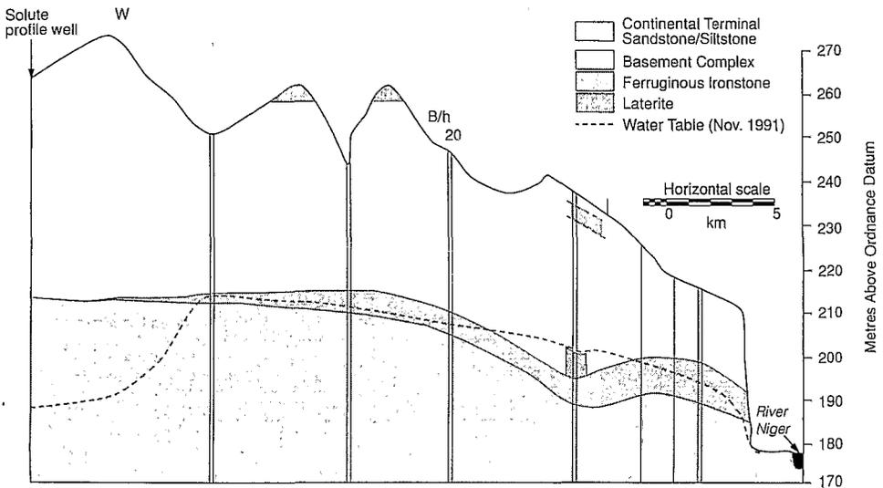
Fig. 1. East-west geological section of the aquifer in the southern bank (see location in Fig. 3).
