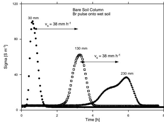
Fig. 3 TDR measured bulk-soil EC
