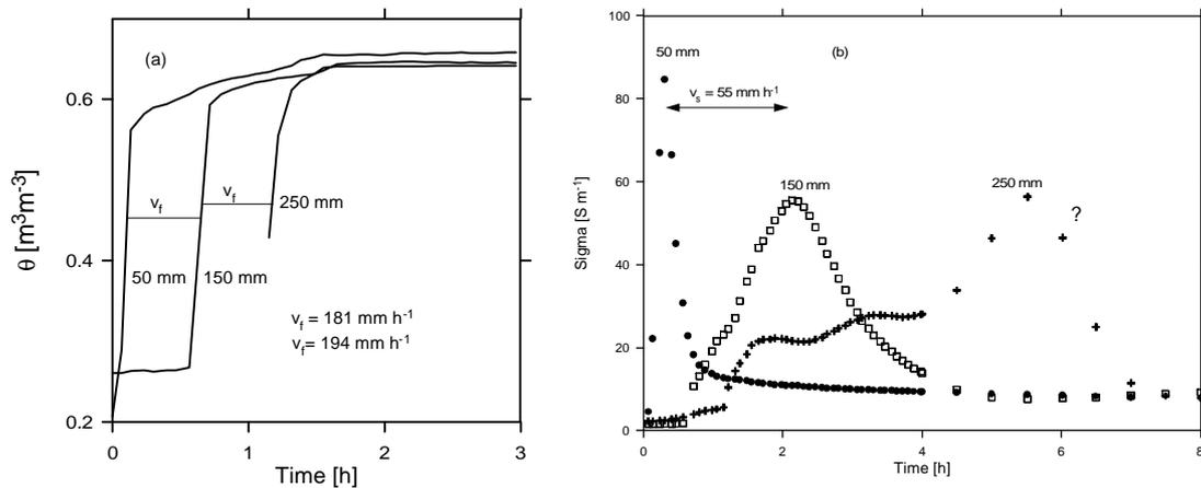
Fig. 5 (a) TDR measured water content and (b) bulk soil electrical conductivity.
