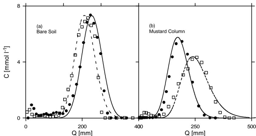
Fig. 1. Measured and predicted BTC's of bromide (● and solid line) and nitrate (□ and broken line).
