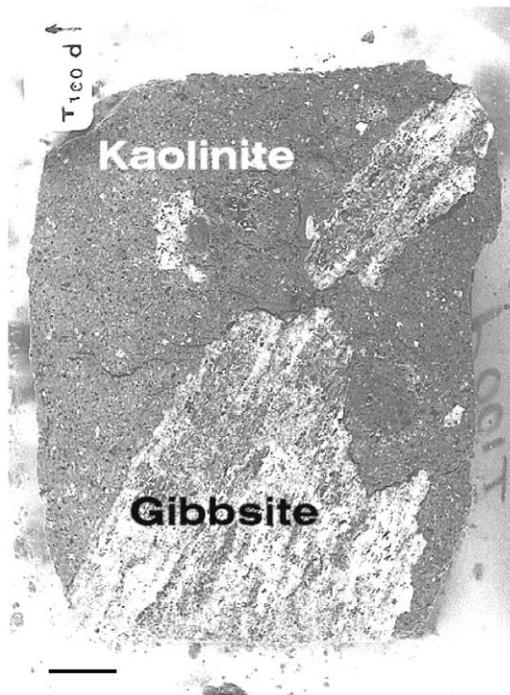
Fig. 7. Detail of the contact between kaolinitic clay loam horizons and gibbsitic saprolite on an impregnated block. Bar = 1 cm.
