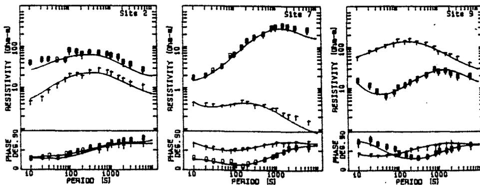
Fig. 2. Examples from two sites (7 and 9) of the tensor resistivity and phase data for the TE (dots) and TM (crosses) directions. At site 2 data represent tensor parameters calculated in a fixed coordinate system which is parallel
