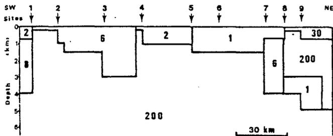
Fig. 4. 2D resistivity model along the Altiplano traverse. Resistivities are given in ohm meters. See Figure 1 for MT site locations.
