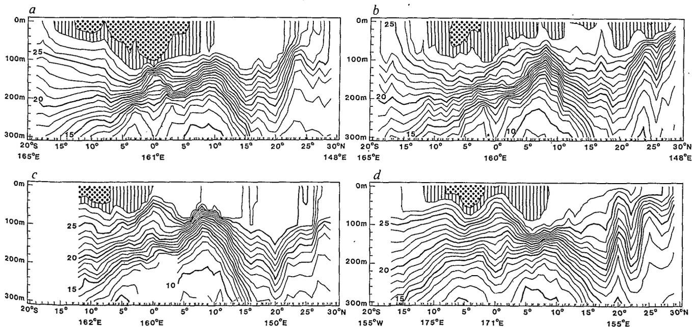
Fig. 1 Meridional temperature sections along the shipping route between New Caledonia and Japan. a, 2-12 January 1982; b, 28 July-7 August 1982; c, 8-17 January 1983; d, 1-21 June 1983. Waters with temperatures exceeding 28 °C and 29 °C are highlighted by stripes and dots, respectively. Station locations are indicated by x at the bottom of each panel.
