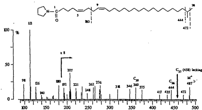
FIG. 4. Mass spectrum of 27-methyl-5,9-octacosadienoic acid pyrrolidide showing the typical fragmentation peak at m/z 180 and lack of a peak at m/z 458 ( C_{27} fragment).
