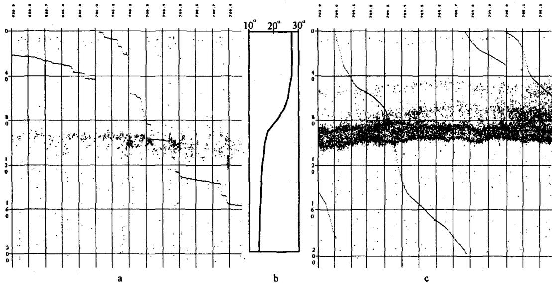
**Figure 6** Typical detection of *Vinciguerria nimbaria* and thermal structure : a/ daylight echogram showing small schools; b/ thermal profile, showing a well-marked thermocline between 60m and 90 m depth; c/ night echogram showing a scattering layer with swarms inside, at the bottom of the thermocline, about the same depth as during daytime.
