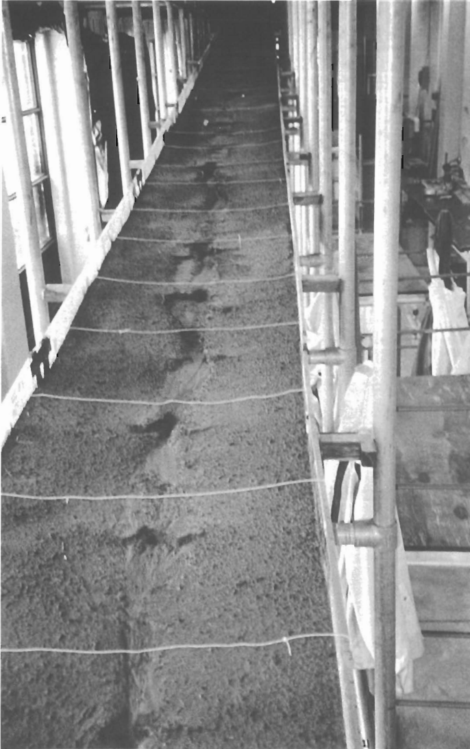
Fig. 5. Multiple sequential scour/deposition cycles formed under simulated rainfall in 22.5 m long laboratory flume.
