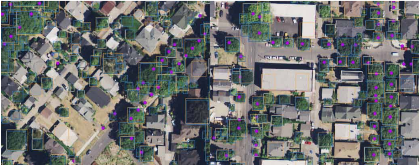
FIGURE 7 Predictions for the Portland street tree case study. Bounding box predictions from the prebuilt model are in orange. Bounding box predictions from the retrained model using local data are in blue. Street tree locations are marked in purple
