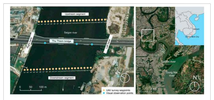
FIGURE 1 | Localization of visual observation points and 22 Unmanned aerial vehicle survey waypoints. Right and left river banks refer to the hand sides when facing downstream. Source: Bing imagery.
