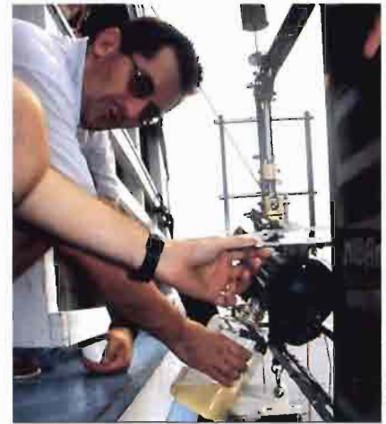
Taking a water sample from CLD-2 sampler coupled with a CTD probe.
