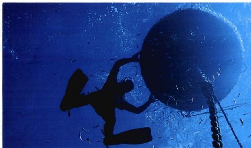
Installing an instrumented buoy (with echo sounder) on a FAD in French Polynesia
