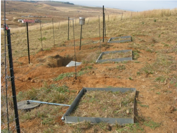
Figure 2a. Installation of the 1m 2 frame on a single contour line in pastures in South Africa. The collection tanks are protected by barbed wire.
