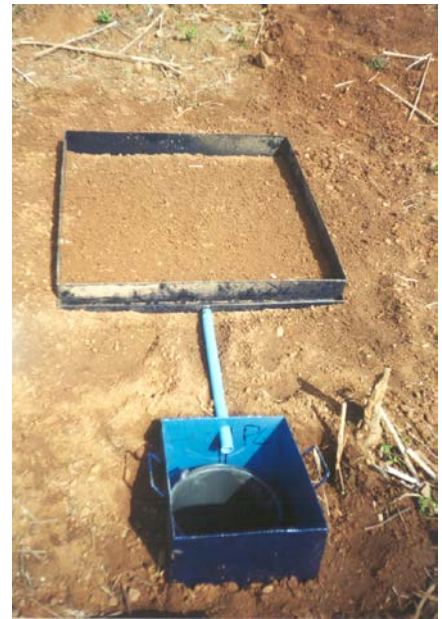
Figure 5b. Plot set-up on crop area. An iron tank was installed to prevent the bucket floating.
