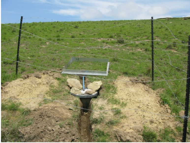
Figure 5a. Plot set-up on degraded grassland in South Africa. A trench drain was dug to prevent the tank floating.
