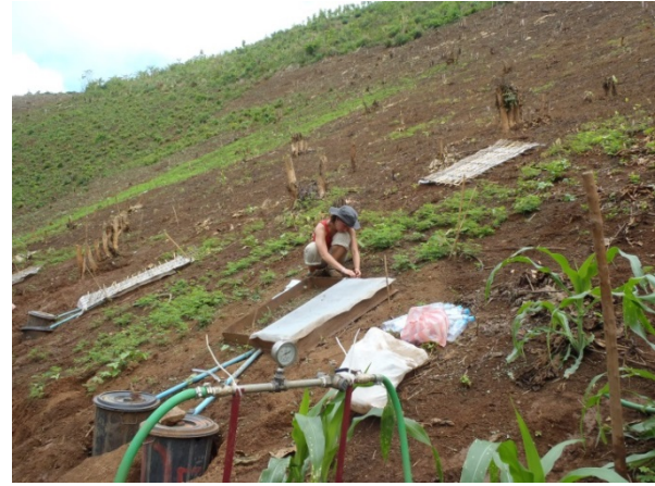
Figure 2b. Installation of the 1m 2 frame on two contour lines in crop area with steep slope in Laos.
