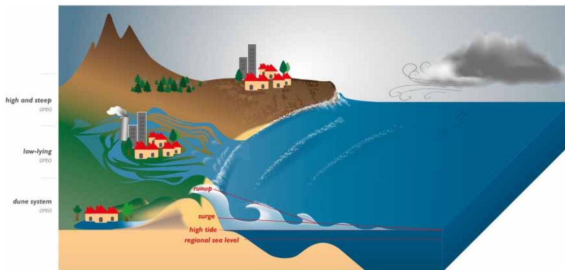
Fig. 1 Schematic of the processes governing coastal overtopping and the different levels of potential flooding depending on coastal topography. The extreme coastal water level (ECWL) results from the combination of regional sea level anomaly (SLA) due to the steric effect, ocean circulation and transfer of mass from the continents (ice sheets, glaciers, land water) to the ocean, astronomical tide ( T ), storm surge due to atmospheric pressure and winds (DAC), and wave runup ( R ), decomposed into a time-averaged component (setup) and an oscillatory component (swash).
