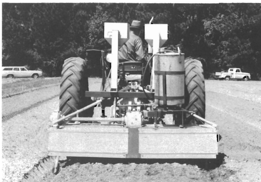
Fig. 8. Liquid and granular applicators for applying non-fumigant nematicides mounted on tractor drawn rototiller for incorporating (Photo: A. W. Johnson).
