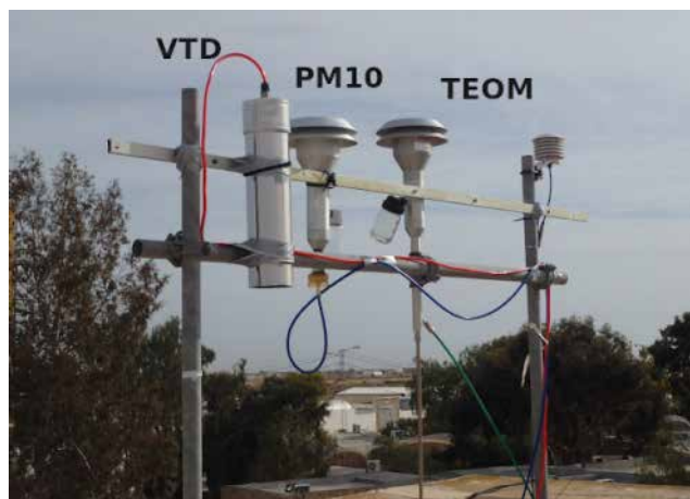
Figure 1. From left to right, the VTD system, the PM 10 sampling head, and the TEOM. Both the TEOM and PM 10 heads are from the same brand: Tecora™ PM 10 .
