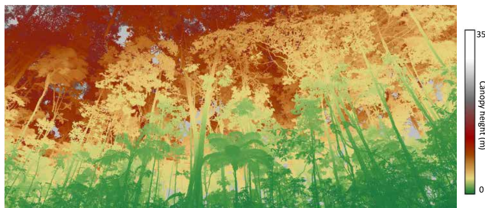
Fig. 1 A view from a Central Amazonian forest understory. Colours depict plants within distinct vertical strata. The high-speed terrestrial laser scanning (TLS) data acquisition of 500,000 measurements per second provides detailed measurements capable of detecting fine-scale changes in vegetation structure. We used a scan resolution of 40 mdeg in both azimuth and zenith directions, which results in a point spacing of 1.4 cm at a 20 m distance from the scanner. The laser pulse repetition rate used was 600 kHz, allowing a measurement range of up to 350 m and up to eight returns per pulse.
