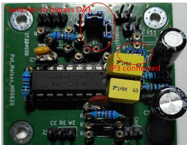
Fig. 6. PassStat 2.0. Ground is deported to 1.65 V thanks to resistors R_9 and R_{10} .
