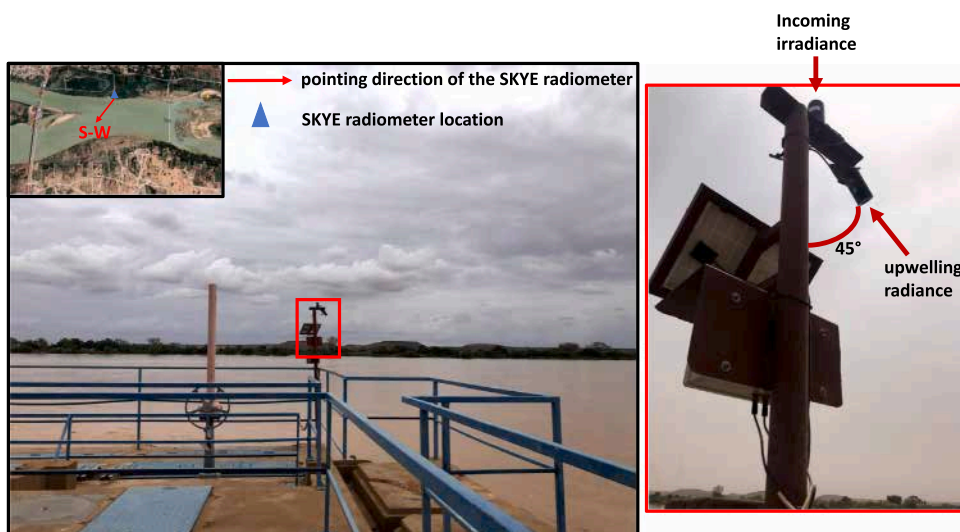
Fig. 3. SKYE radiometer at the Sampling station monitoring Niger River water reflectance.
