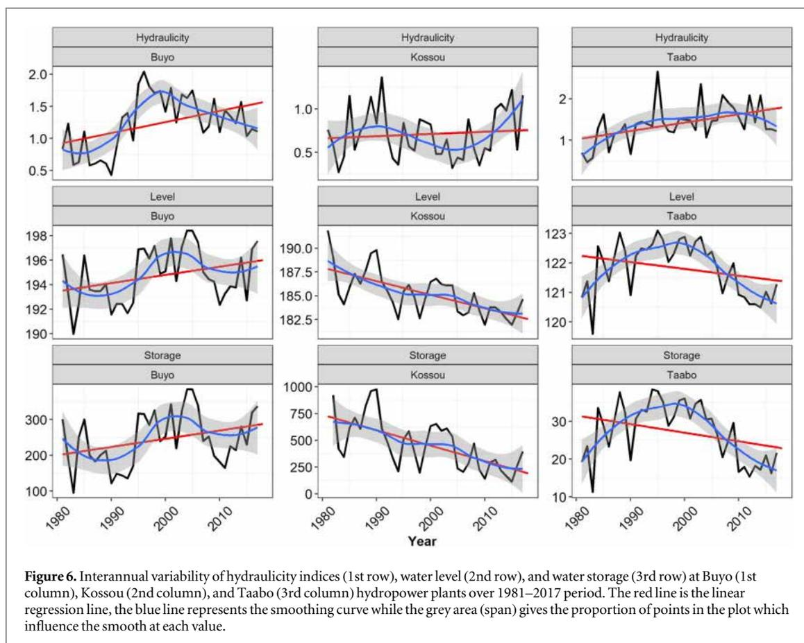
**Figure 6.** Interannual variability of hydraulicity indices (1st row), water level (2nd row), and water storage (3rd row) at Buyo (1st column), Kossou (2nd column), and Taabo (3rd column) hydropower plants over 1981–2017 period. The red line is the linear regression line, the blue line represents the smoothing curve while the grey area (span) gives the proportion of points in the plot which influence the smooth at each value.
