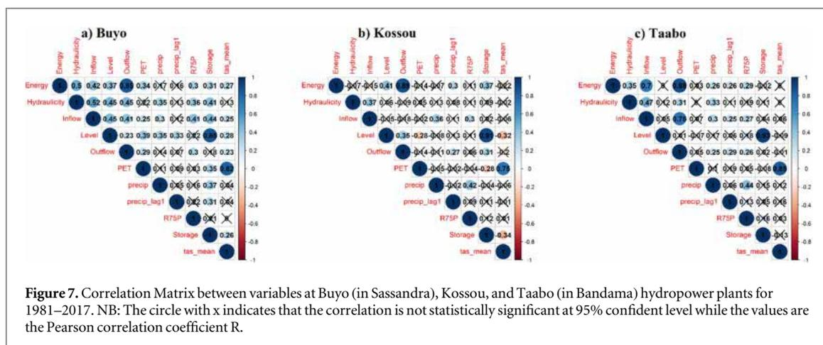
**Figure 7.** Correlation Matrix between variables at Buyo (in Sassandra), Kossou, and Taabo (in Bandama) hydropower plants for 1981–2017. NB: The circle with x indicates that the correlation is not statistically significant at 95% confident level while the values are the Pearson correlation coefficient R.
