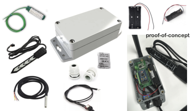
Figure 2. The INTEL-IRRIS soil sensor device.
