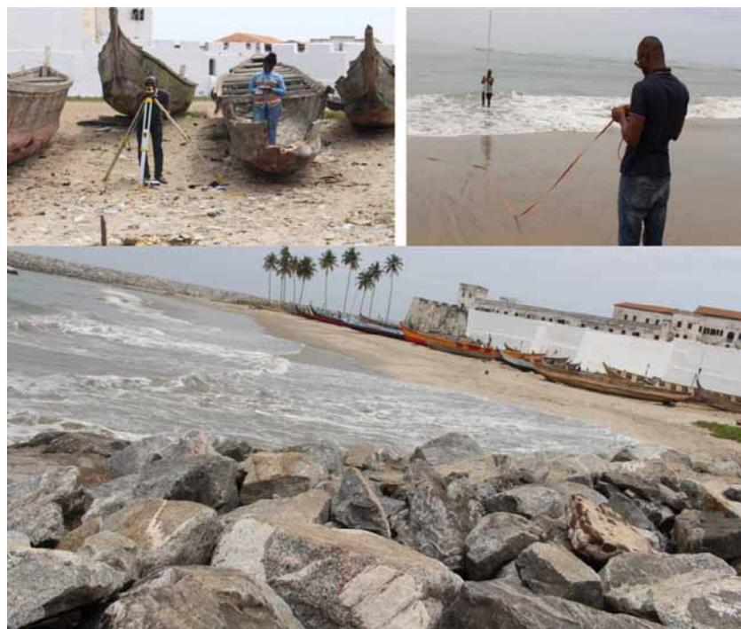
Fig. 2. Beach profile measurements in front of the Elmina Castle using a dumpy level.
