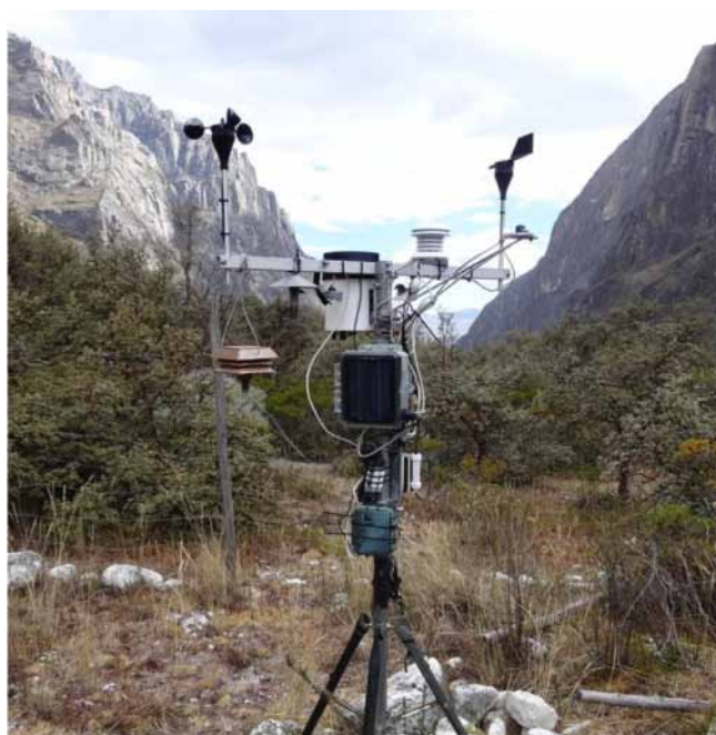
Figure 3. The typical setup for the HOBO automatic weather station; shown here is the LlanWX station near the lower lake in Llanganuco. Measurements include air temperature, humidity, wind speed and direction, incoming solar radiation, and rainfall. Note also the two Lascars with different radiation shields hanging from the crossbar. Photographs taken by Robert Hellström (Covert, 2016).
