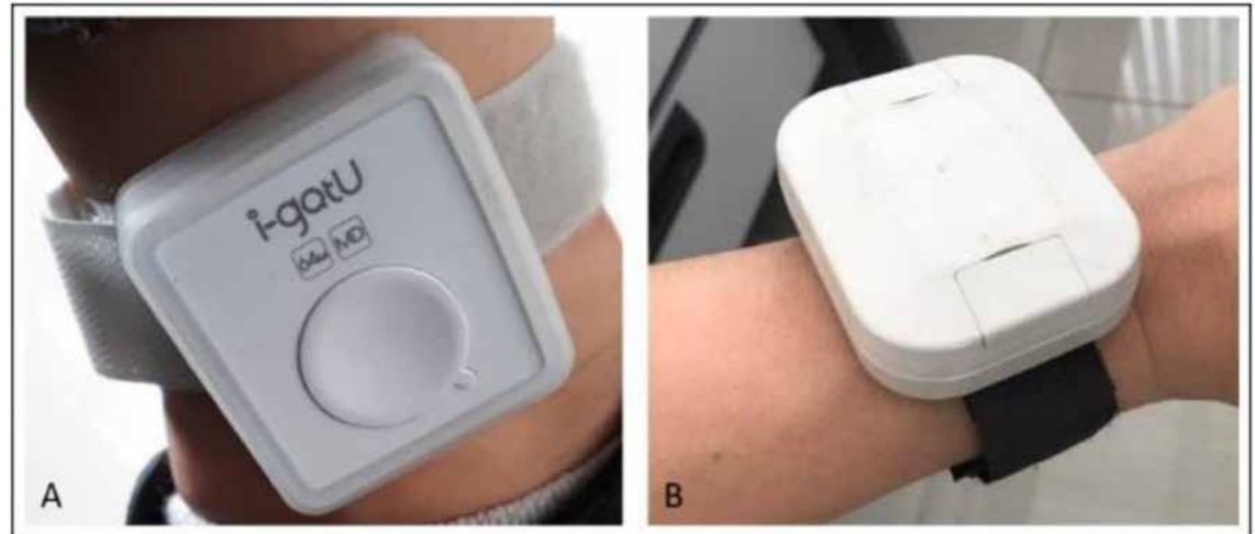
Fig 1. Devices distributed to the study population. A: I-gotU GT600, distributed for rainy season (here worn on an individual's ankle), B: Takachi waterproof enclosure containing the I-gotU GT600 distributed for dry season (here worn on an individual's wrist). The waterproof enclosure was not yet used during rainy season because the devices were sold as "water-resistant" and were expected to be adapted to study conditions.
