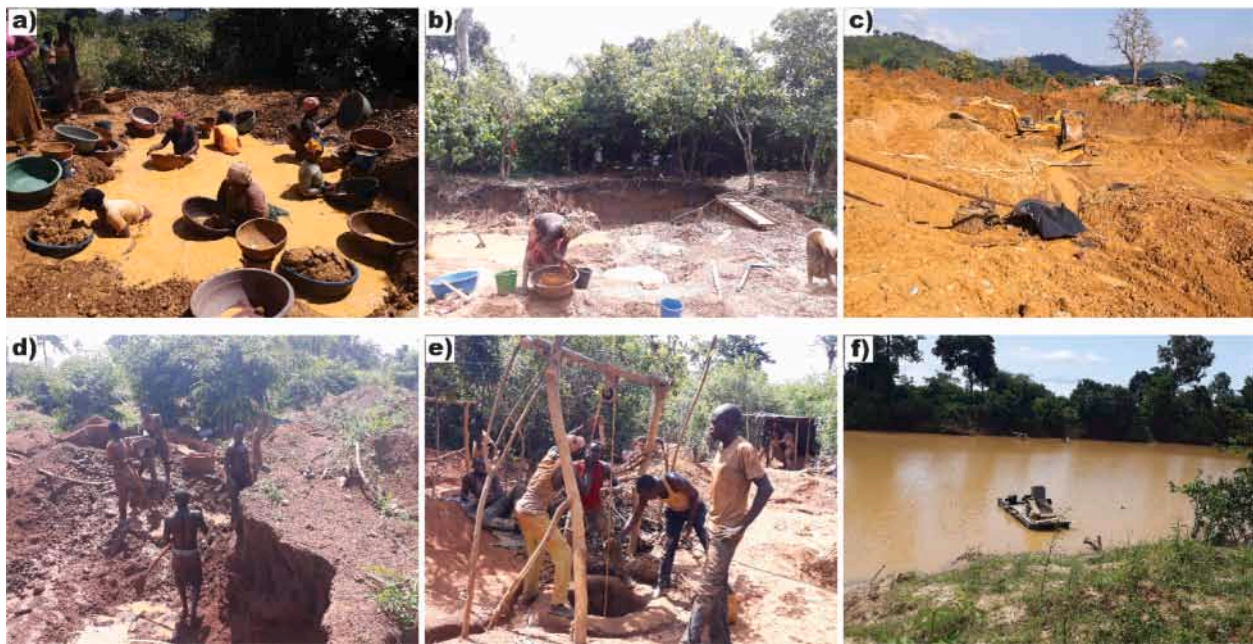
Fig. 3. Artisanal mining sites visited during the field work. (a & b) women washing ore in Kaoukougnanou, (c) semi-industrial exploration in Angovia, (d) exploitation of duricrust levels rich in gold in Kavyessou, (e) extraction well, (f) the brown color of the water of the Bandama river illustrating its important sediment load.
