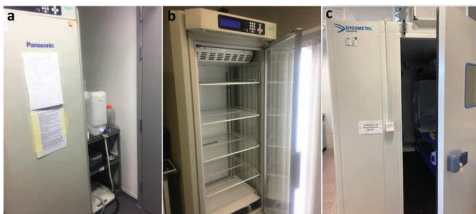
Figure 3. Examples of environmental/climatic chamber with humidity, temperature, and light control. (a, b) Climatic chamber connected to a water container for water supply and to a waste container to collect wastewater. (c) Walk in climatic chamber.
