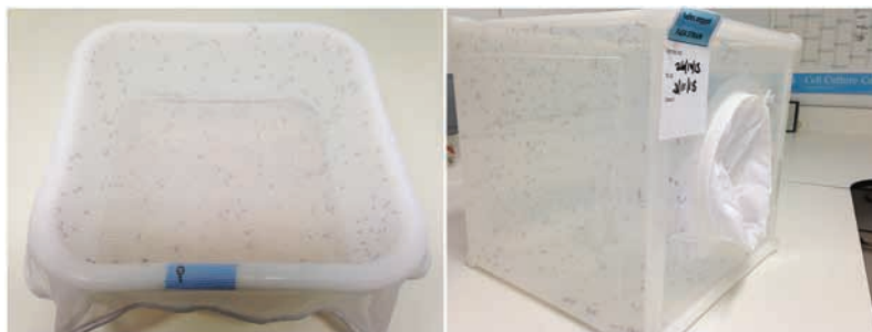
Figure 5. Primary containers for non-infected mosquitoes. Left panel, breeding pan covered with a weighted net for mosquito larvae. Adults can emerge in pans and are further aspirated. Right panel, typical cage for adult mosquitoes with plastic and meshed panels plus a mesh sleeve allowing access.
