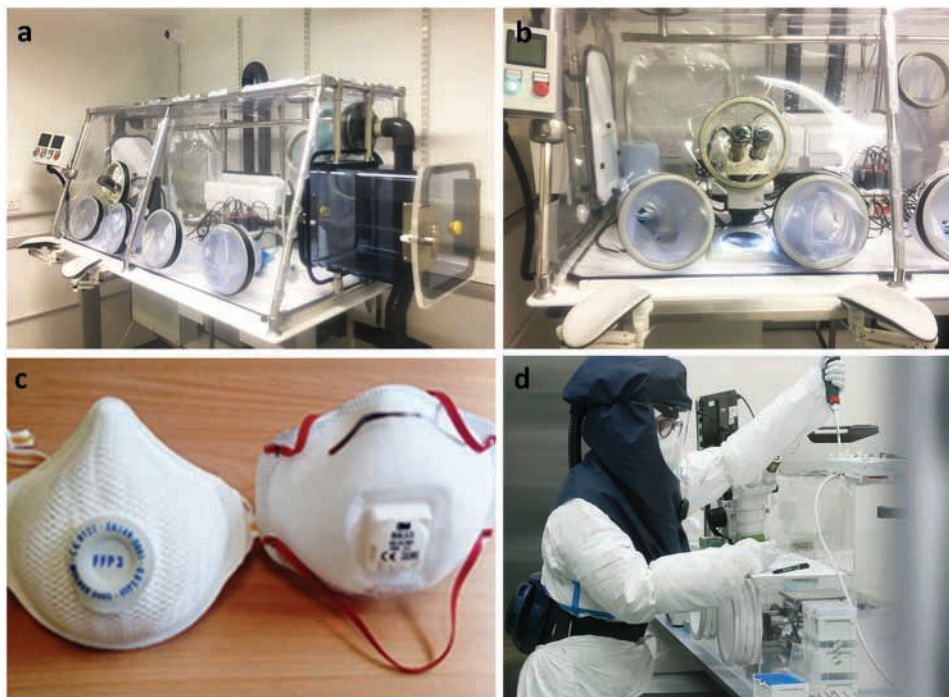
Figure 11. Protective equipment to work with HG3 pathogens. (a) HEPA-filtered isolator working under negative pressure for manipulation of HG3 infectious material which can be aerosol transmitted. A hatch allows material entry while work is ongoing. Height is adjustable. (b) Incorporated stereomicroscope to dissect infected mosquitoes in HEPA-filtered isolator. (c, d) Filtering face piece (FFP) 3 masks or Purifying Air Powered Respirators (PAPR) that can be used in CL3 in place of a HEPA-filtered isolator.
