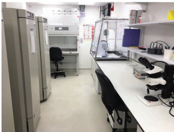
Figure 6. Example of CL2 insectaries dedicated to mosquito infection with HG2 arboviruses. The room is equipped with a class II MSC, to prepare the infectious blood and blood capsules, a glove box, which is a sealed container allowing user to manipulate flying arthropods inside the box without breaking containment, a bench with stereomicroscopes for mosquito dissection, environmental chambers, a freezer to freeze all solid waste before taking out for autoclaving, a sink to dispose of chemically inactivated waste, a UV light trap, a fridge and storage shelves/furnitures.
