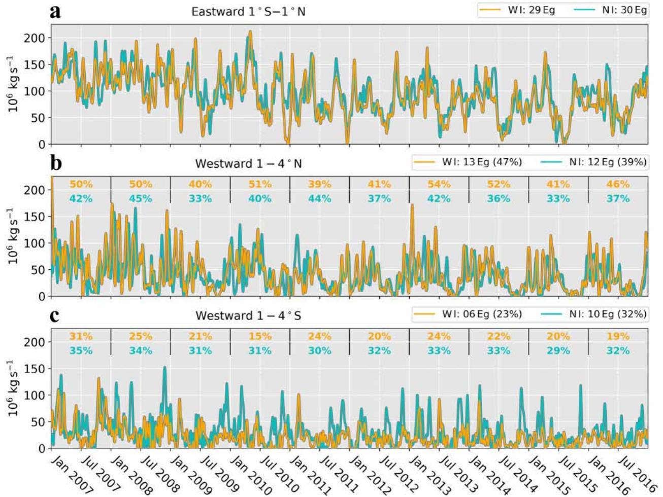
Figure 6. Low-pass filtered (7 days) daily salt fluxes at 4.5^{\circ}\text{E} for the (a) eastward-flowing Equatorial Undercurrent between 1^{\circ}\text{S} and 1^{\circ}\text{N} , (b) Northern Hemisphere westward return flow between 1 and 4^{\circ}\text{N} , and (c) Southern Hemisphere westward return flow between 1 and 4^{\circ}\text{S} . Orange lines represent the With Islands simulation, and cyan lines represent the No Islands simulation. The legend boxes show the integrated transport for the 10-year model series in Eg, (exagram = 10^{15} kg), with yearly percentages of westward transport (b, c) relating the transport in each hemisphere to the total eastward transport at the Equator for the period.
