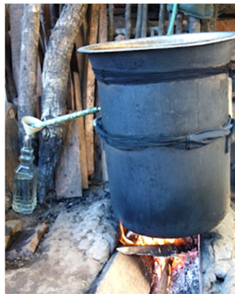
Figure 2. Traditional alcohol production device still in use in the Sayaboury province of Laos.
