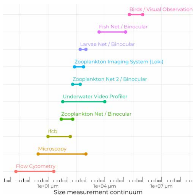
Figure 9. Schematic of the biological sampling size continuum across the various methods and tools used during the Green Edge cruise.
