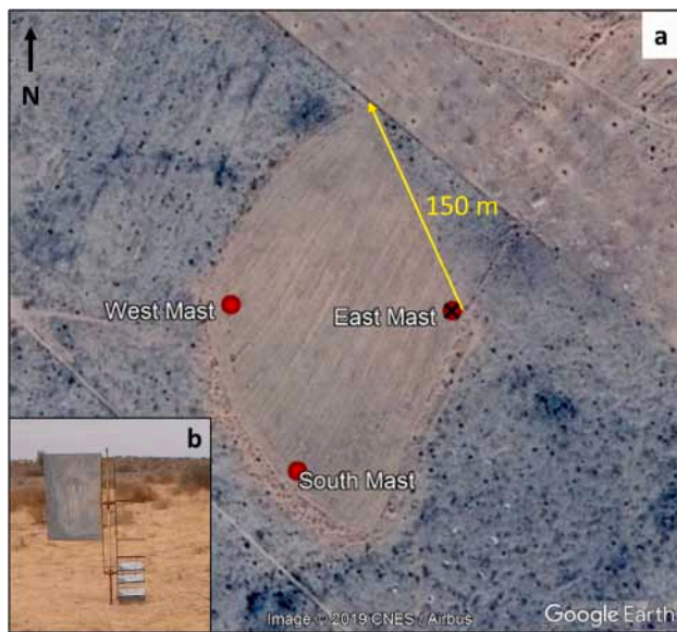
Fig. 1. (a) Google Earth Image (on 27/02/2016) of the experimental plot. Red dots locate the three masts equipped with BSNEs (b). The black cross locates the meteorological masts. (For interpretation of the references to colour in this figure legend, the reader is referred to the web version of this article.)
