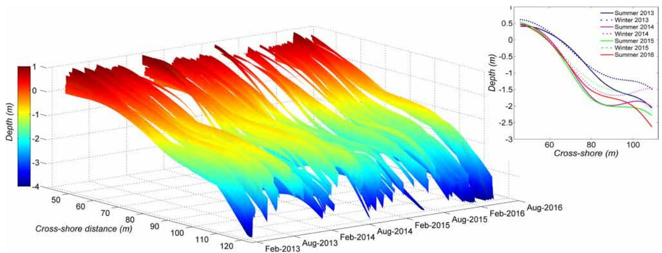
**Figure 5.** Combined intertidal topography and bathymetry profile obtained by processing data from the video camera system installed in Grand Popo, Benin, between February 2013 and August 2016. The upper right panel shows the average profiles over the seasons/years. The figure was generated using *MATLAB R2013a (8.1.0.604)* software.
