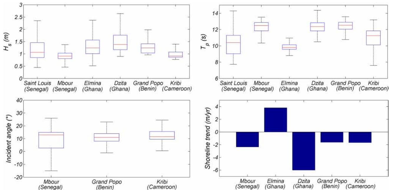
**Figure 3.** Wave characteristics (significant wave height  $H_s$ , peak period  $T_p$  and incident angle to shore) and interannual shoreline trend derived from the African coastal camera network. The figure was generated using *MATLAB R2013a (8.1.0.604)* software.
