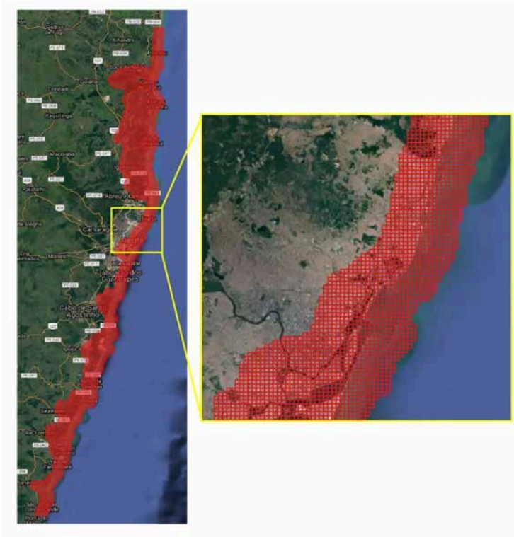
Figure 1. Discretisation grid (in red) of the Pernambuco study area and a zoom on Recife (yellow rectangle)
