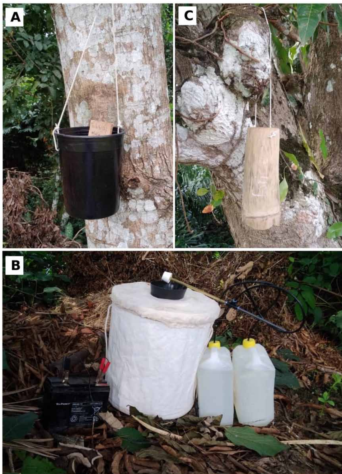
Fig 2. Sampling methods, including plastic ovitrap (A), BG-sentinel trap (B), and bamboo ovitrap (C).
