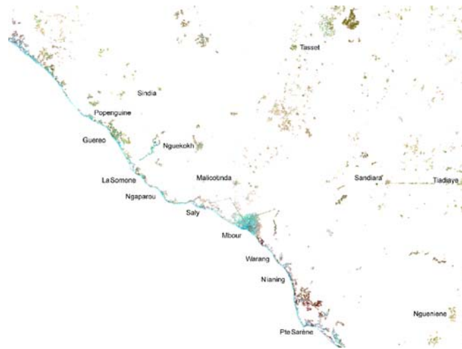
Figure 9. Evaluation of preliminary result by the superimposition of the binary image obtained from reconstruction and the original false colour composition. Example shown for 1988 scene.
