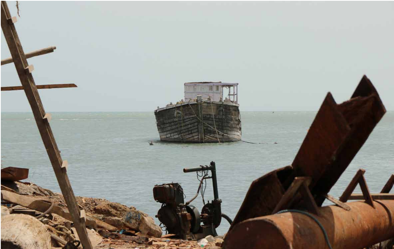
An abandoned thoni is used as an anchor to help in the launching process at Tuticorin.
