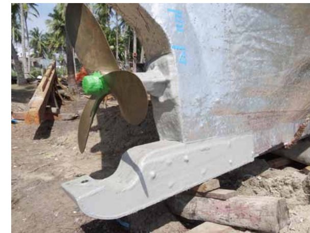
A steel projection is provided to avoid entangling fishing nets in the propeller.
