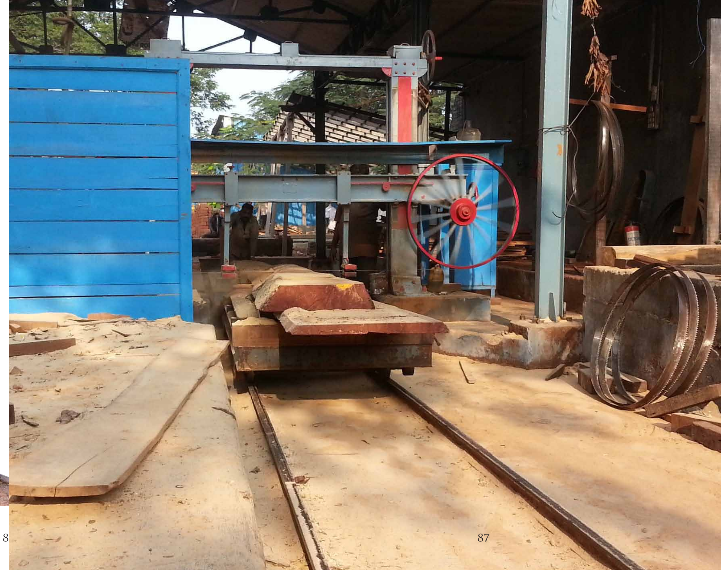
Wooden log of broad diameter is being cut into planks at a timber depot in Pondicherry for a kotia. The Malaysian Sal was imported through Tuticorin.
