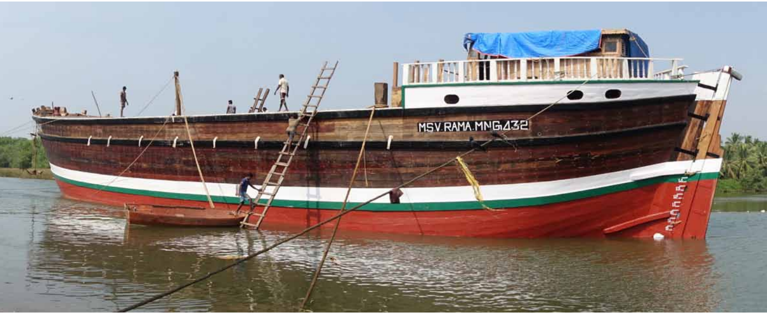
A 400 ton kotia is modified into a 1000 ton vessel destined for Gulf trade, by adding more frames elongating its length.
