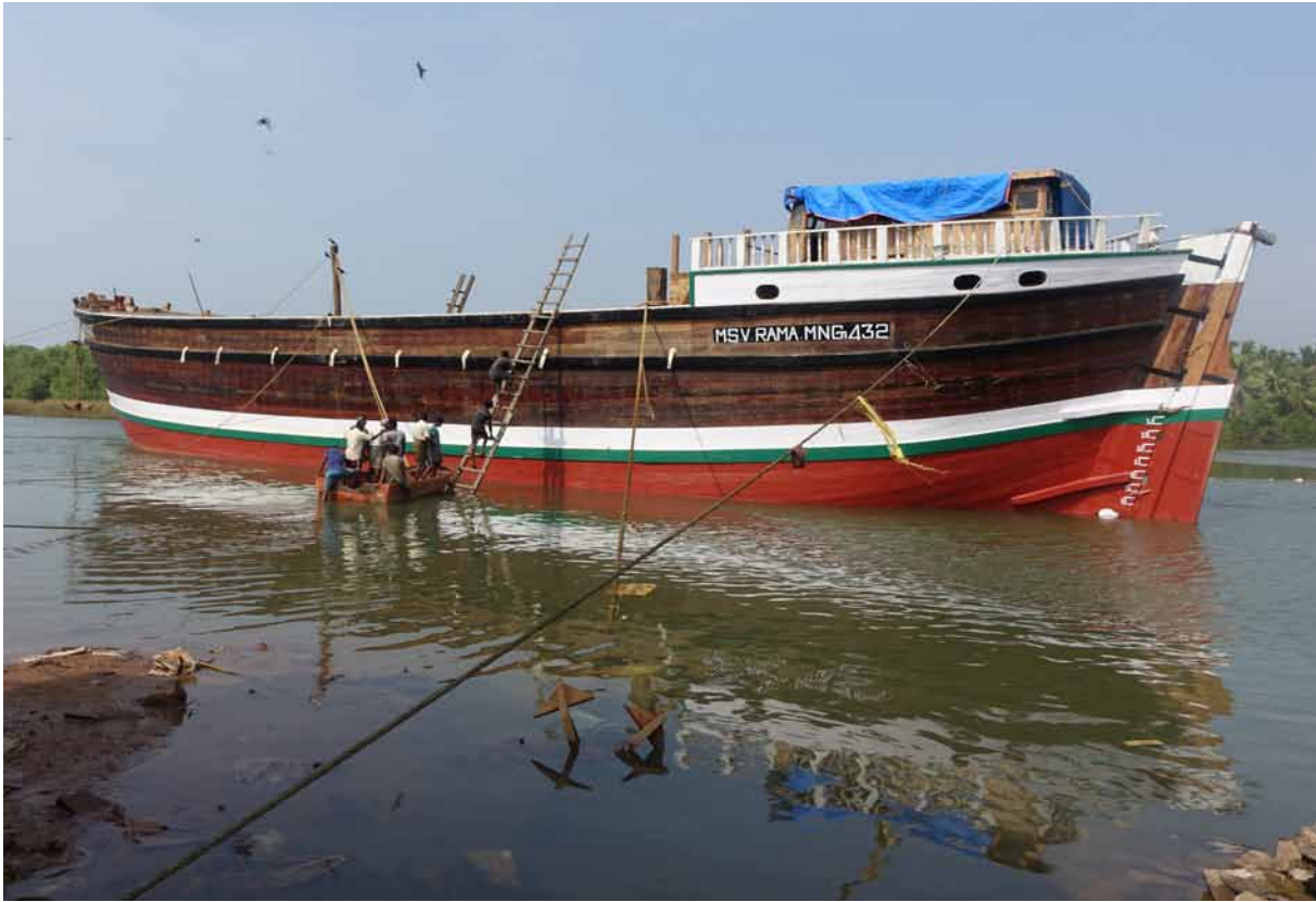
A 1000 ton kotia, extended from a 400 ton by Balu Mistry of Thaikkal on the West Coast for trading in the Persian Gulf, 2015.
