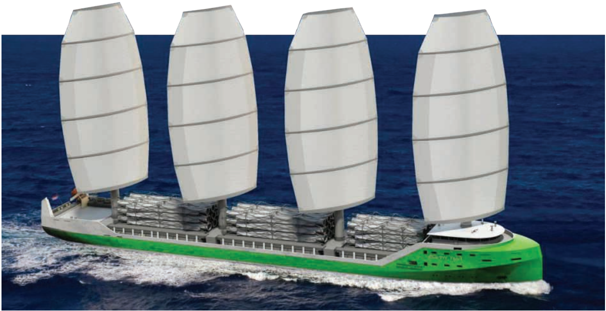
Below: The ecoliner: an example of the new sort of hybrid ships using both sails and motors which are planned nowadays but are still at the stage of concept, unfinished projects or pure prototypes.
