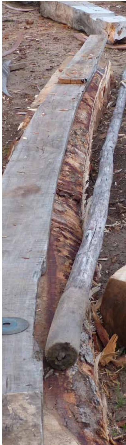
Fig 12d: The completed outline is used to cut the shape of the top frame.
