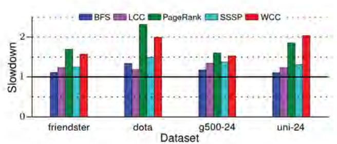
Figure 8: Slowdown when using an iterator interface instead of direct memory access.
