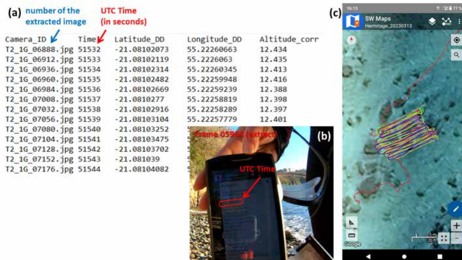
Figure 6. (a) Extract of a five-column file generated by a Python script, comprising the name of the extracted frames, the UTC time and the GNSS positions of the cameras (corrected of the \Delta H offset). This file is then used as Reference file in Agisoft Metashape . (b) Image of the Smartphone filmed by one of the GoPro cameras to capture the GPS time on the SW Maps interface for GNSS-camera synchronisation. (c) Capture of the SW Maps interface for real-time GNSS-camera trajectory tracking (here, on the repeated surveys of the same area in the Hermitage backreef zone, on 13 March 2023).
